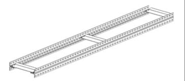
**5.** With the help of an associate, raise one EUR upright set (from starter unit) and the ZTP upright set and connect them with left to right channel beams (Ref. No. 3). Be sure the channel beams are fully seated.
