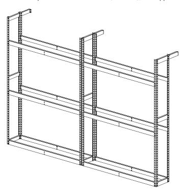
NOTE: Wall Ties are REQUIRED to be used for unit stability on Single Entry Units.
