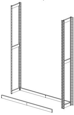
**6.** Continue to build your shelf levels by placing left to right channel beams at the desired locations.
