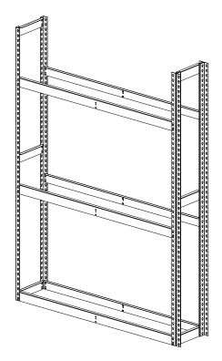
**7.** With the help of an associate, raise the remaining EUR upright set (from starter unit) and the ZTP upright set and connect with left to right channel beams Be sure the channel beams are fully seated.
