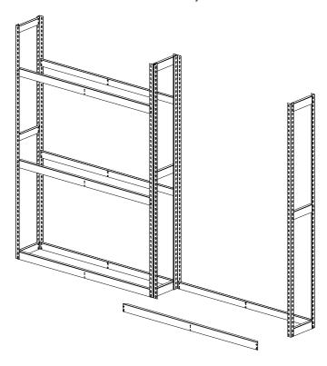
**8.** Continue to build your shelf levels by placing left to right channel beams at the desired locations.
